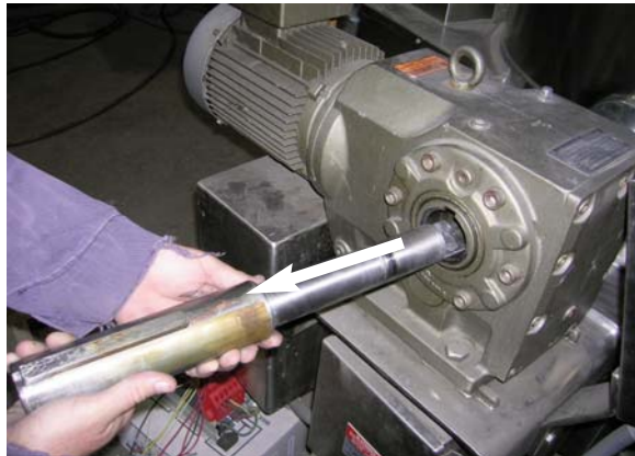
5. Gently hammer out shaft and remove.
